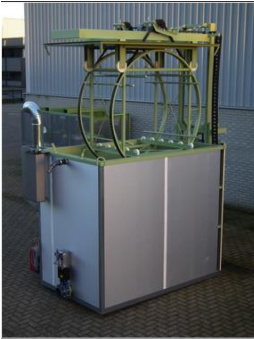
Figure 8. Akerboom's box sterilising apparatus. Built to client specifications
